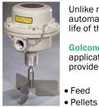
Unlike many other available paddle units Golconda's paddle level indicators incorporate a feature that automatically shuts off the motor of the unit when the paddle is in a stalled position, which both extends the life of the motor and minimizes maintenance.
